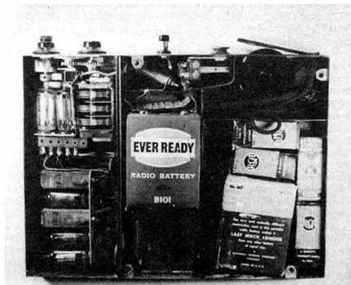
A compact "briefcase" superhet receiver with room for spare battery, spare valves and earphone, yet still a thin unit. Believed to have been a "Whaddon Special" for Intelligence operations about 1943-4. (Photo: Keith Melton, USA)
